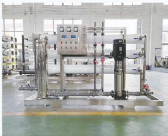
HC-RO-5T~10T/时反渗透设备
